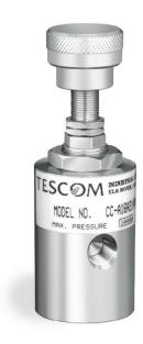
TESCOM CC Series metering valve is rated to 10,000 psig / 690 bar and contains a non-rotating stem to reduce seat and stem wear. The valve features over 20 turns from shutoff to full open, providing excellent flow control.
